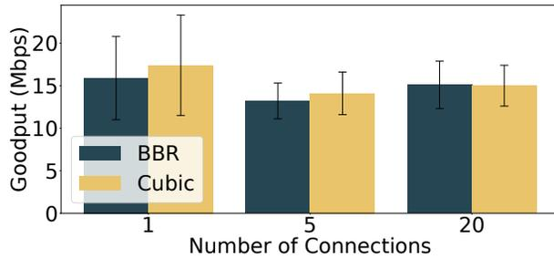
**Figure 9: The goodput of BBR under Low-End configuration over cellular. BBR and Cubic performance is similar under all settings (unlike results over WiFi and Ethernet where Cubic outperformed BBR.) We find that this is because in cellular networks, the setting is bandwidth-limited and not CPU capacity-limited.**
